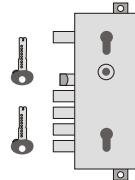
Cylinder gear lock with anti-tampering trap
